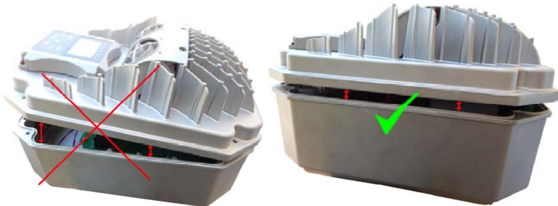
Please make sure, the motor terminal box has enough mechanical stability to support the inverter
